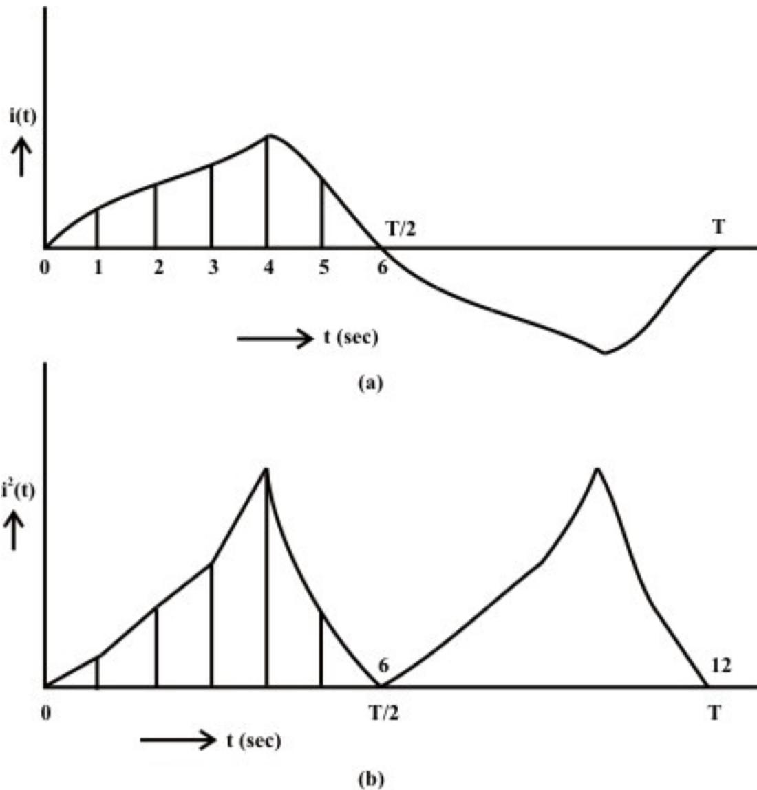
**Fig. 12.3 Periodic current waveform**
