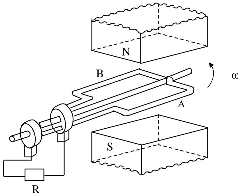
**Fig. 12.1 Schematic diagram for single phase ac generation**
