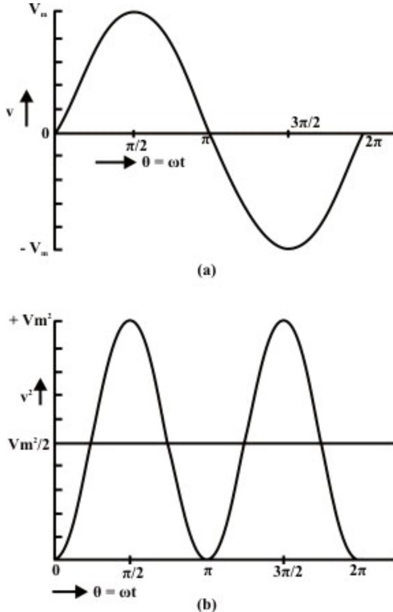
**Fig. 12.4 Sinusoidal voltage waveform
